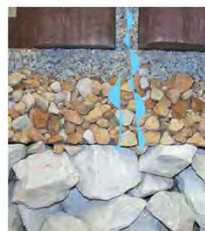
Permeable interlocking concrete pavement (PICP) with base and subbase for infiltration and storage
